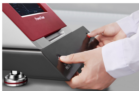
Lever Clamps hold the sample securely for making the initial cut and for testing.
