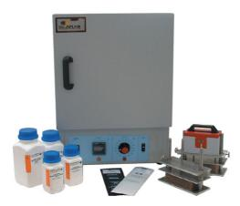
To determine colorfastness to water and perspiration of textiles. Provided with 2 stainless steel frames each with a capacity of 20 samples of 10 cm  $\times$  4 cm held between acrylic separator plates. Loading weights for BS, ISO and AATCC standards are included. An electric incubator is required available but not included.
