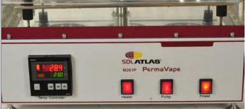
The test station platform is easily adjustable to ensure that the samples are immersed to the proper depth in the bath.
