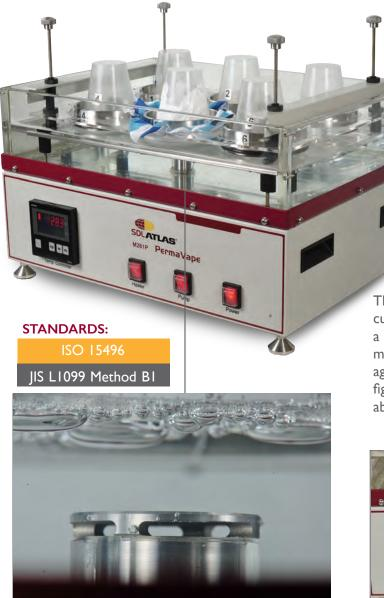
The water bath is heated to the required temperature of  $23^{\circ}$ C and maintained evenly throughout the bath through a circulation pump.
