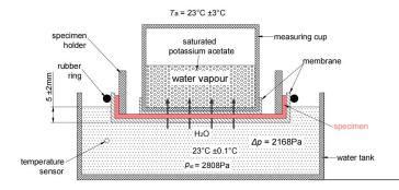
The user-friendly **Perma-Vape** delivers accurate and reliable results for water vapor permeability.
